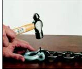
2. Place the coupler link on its side and using a hammer, drive the locking pin into the clevis ear until it is flush with the outside surface.
