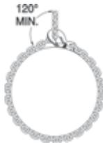
In shortening applications, a 20% reduction of the Working Load Limit is required except when using the Crosby A-1338 Cradle Grab Hooks, S-1311 Chain Shortener Link, the A-1355 Chain Choker Hook in conjunction with the S-1325 Chain Coupler Link, or the Crosby ELIMINATOR® shortener link. They can be used without any reduction to the Working Load Limit.
