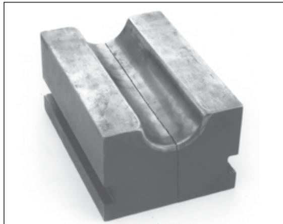
**Never use dies that are cracked, worn or abraided (galled).**
