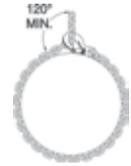
In shortening applications, a 20% reduction of the Working Load Limit is required except when using the Crosby A-1338 Cradle Grab Hooks, S-1311 Chain Shortener Link, the A-1355 Chain Choker Hook in conjunction with the S-1325 Chain Coupler Link, or the Crosby Eliminator® shortener link. They can be used without any reduction to the Working Load Limit.
